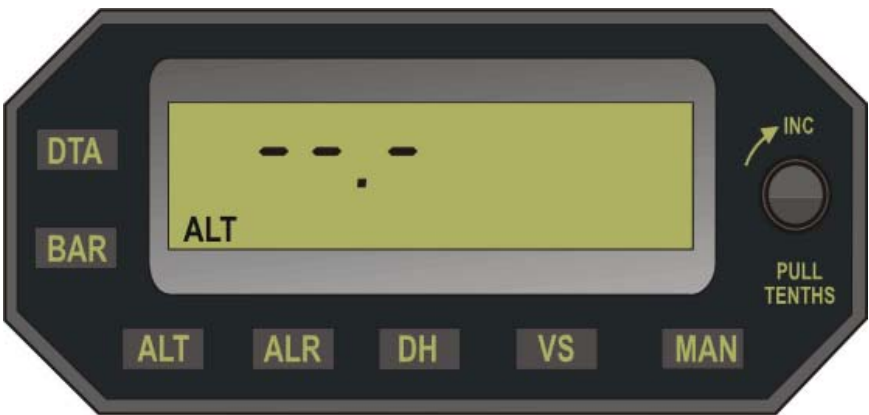
Fig. 3-1. Selector / Alerter Display, Loss of Encoded Altitude
